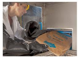
An operator transfers empty bags from the glove box side of the enclosure through a bag infeed chute in the enclosure sidewall, drawing dust generated from bag compaction as well as dumping activities into the integral dust collection system.
