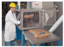
The operator is isolated from dust by means of a dumping hood comprised of a plastic strip curtain, glove box, empty-bag infeed chute, and dust collector atop a receiving hopper feeding an enclosed flexible screw conveyor.
