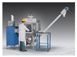
Dust generated from bag opening, dumping and compaction is isolated from the operator and plant environment by means of a glove box, dust collector and integral bag compactor with sealed infeed chute. An enclosed Flexicon flexible screw conveyor transfers material downstream at any angle, dust-free.
